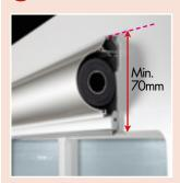
The height must be at least 70mm in the upper section, measuring upward from the molding, so that the box is not visible behind the door (flat surface).
