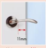
Minimum space of 11mm between the doorknob and the edge of the inner molding (as long as the surface is flat).
