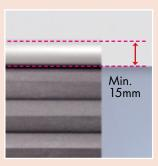
The height must be at least 15mm in the upper section, as measured from the molding upward (flat surface).
